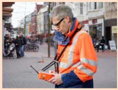
Figure 3: Pinpointing the leak with a correlator
